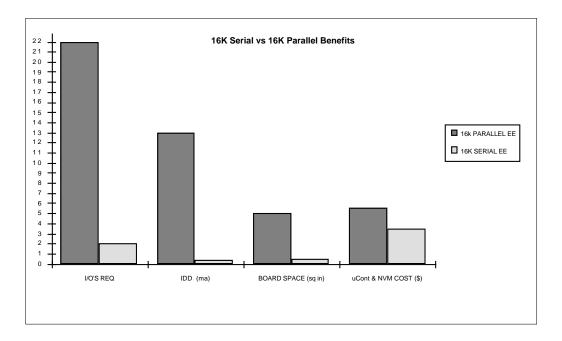
The Serial EEPROM requires only 10% of the board space that a Parallel EEPROM requires. Also, the Serial EEPROM requires fewer I/O lines from the microcontroller which significantly reduces the overall system cost and board space.
